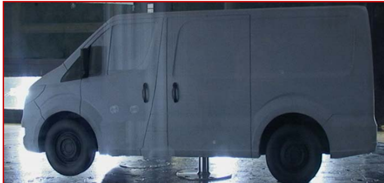
Drag reduction study on a truck model
