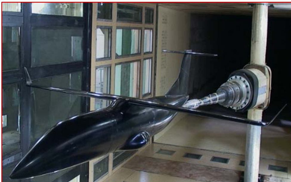
Aircraft model mounted on Robotic Arm for aerodynamic study
