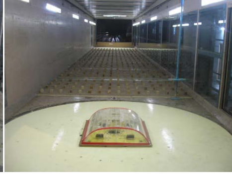
Model of industrial curved roof
