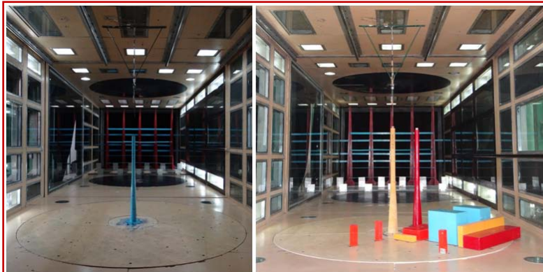
Chimney model studied under stand-alone and interfering conditions
