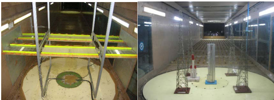
Sectional models of bridge decks
