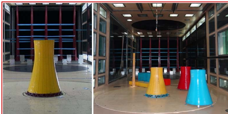
NDCT model studied under stand-alone and interfering conditions
